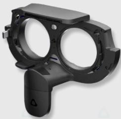
**VIVE Full Face Tracker** is a plug-and-play USB-C module that enables detailed face and eye tracking on compatible devices. It captures 38 facial blend shapes at 60 Hz and tracks eye movements at 120 Hz, allowing for natural expressions and real-time lip-sync. It also auto-calibrates Interpupillary Distance (IPD) for optimal comfort and clarity.
