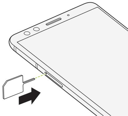
When inserting the eject tool into the tray eject hole to remove the card tray, do not obstruct the tray to avoid damaging the eject mechanism inside the slot.
