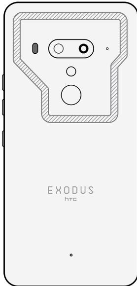
Make sure that the NFC area (shaded part) of HTC EXODUS 1 and the other phone's NFC area are close to one another. Experiment by slightly moving the phones until a connection is made.
