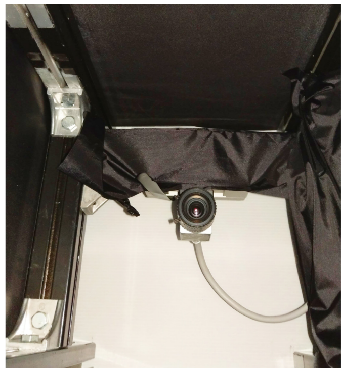
CCD camera modules dismantled from old jigs are applied 100% on new project stations, and are re-designed as new equipment.
