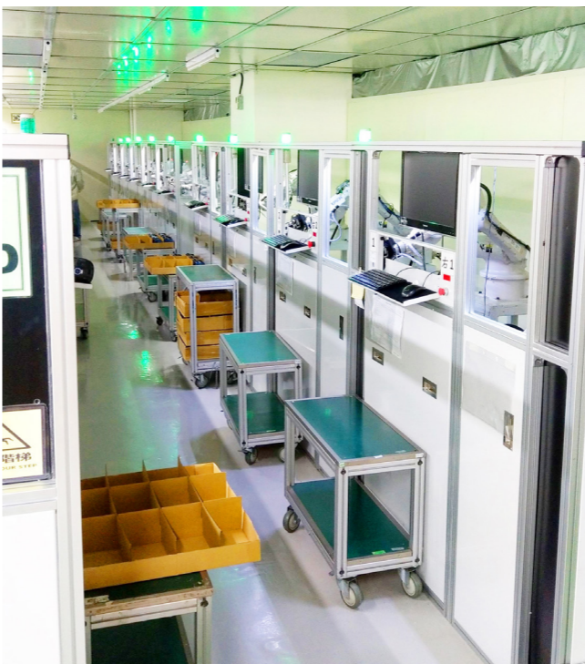
Aluminum extrusion and recycled materials dismantled from old project stations are re-assembled as new ones.
